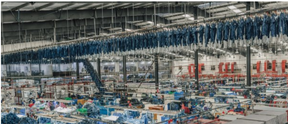
Figure 6: Air drying method for the denim products using air recycled from hot factory machinery
