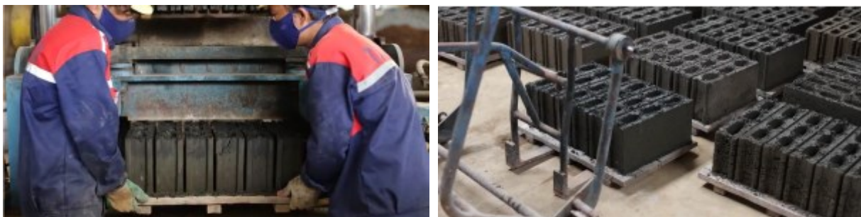
Figure 7: Bricks created by mixing the sludge, the toxic waste of the denim process
