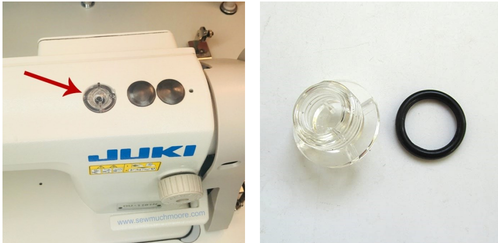
Figure 3. Sight window to see a flow or splash of oil
